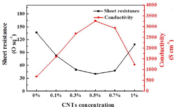
Fig. 2. Electrical properties of PEDOT:PSS films with different CNTs concentration
