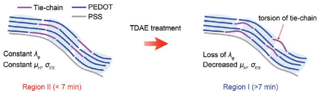
Fig. 3 Schematic illustration depicting the change in structural connectivity by tie-chain torsion in PEDOT:PSS after 7-min duration of de-doping. The tie-chain torsion degrades the charge transport between crystalline domains.
